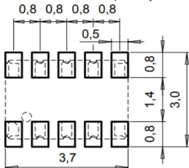
Tolerances: unless otherwise specified  $\pm 0.1\text{mm}$
