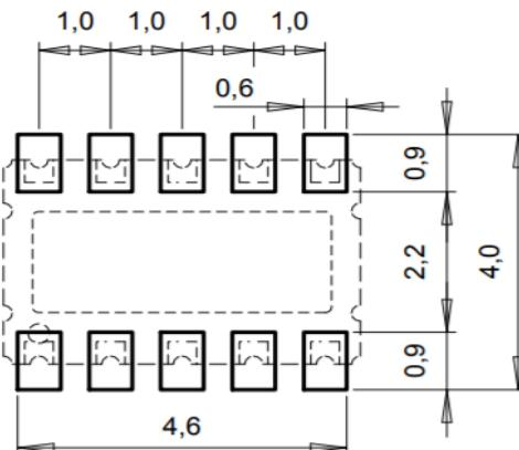
Tolerances: unless otherwise specified  $\pm 0,1\text{mm}$
